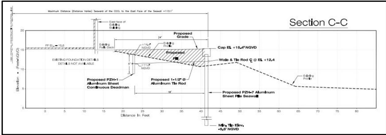
Figure 1a – Typical Cross-Section: Seawall with Tie-rod & Deadman
