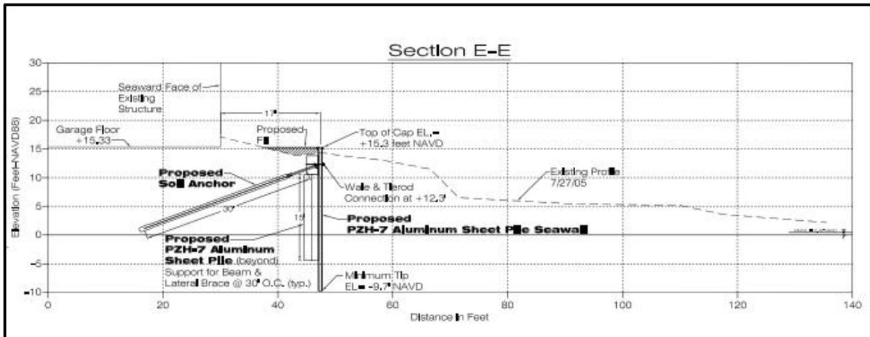
Figure 1b – Typical Cross-Section: Seawall with Soil Anchor
