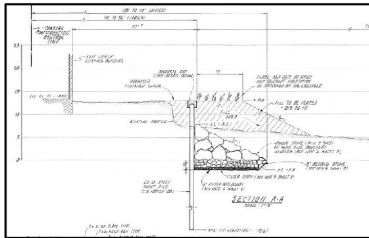
Figure 1c – Typical Cross-Section: Cantilever Seawall with rock toe-revetment
