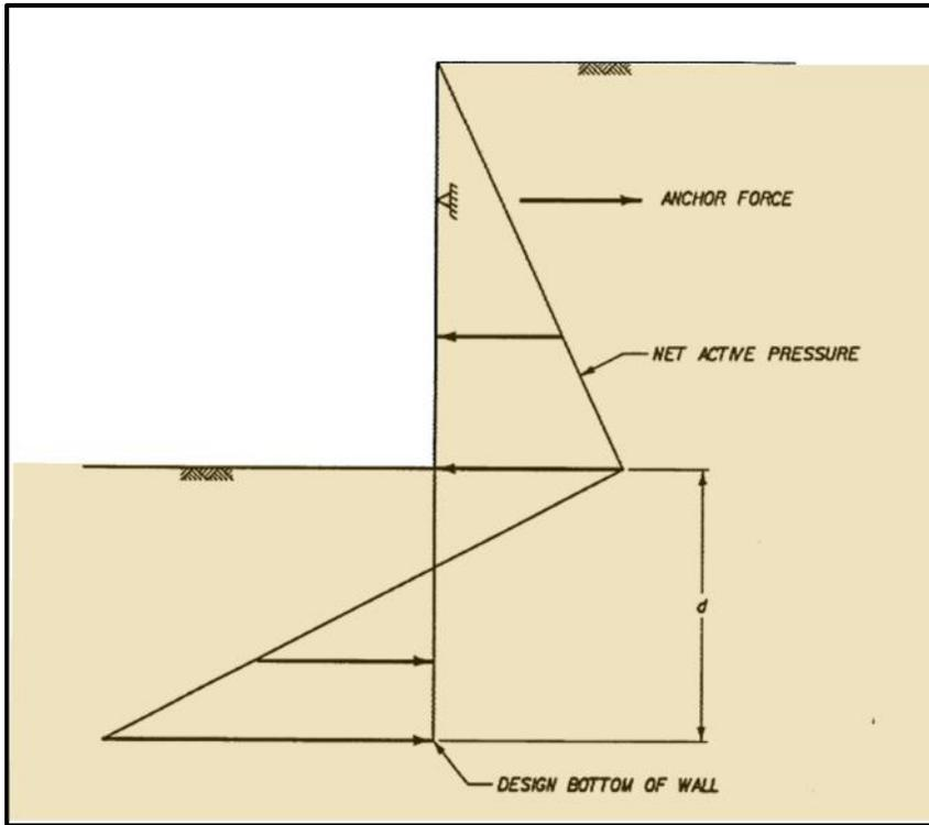
Figure 2a – Laterally Restrained Seawall - with Anchor
