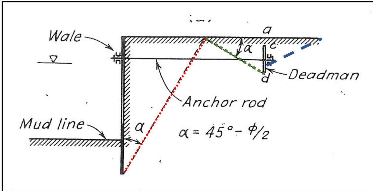
Figure 3 – Failure Planes (adapted from Peck et al)
